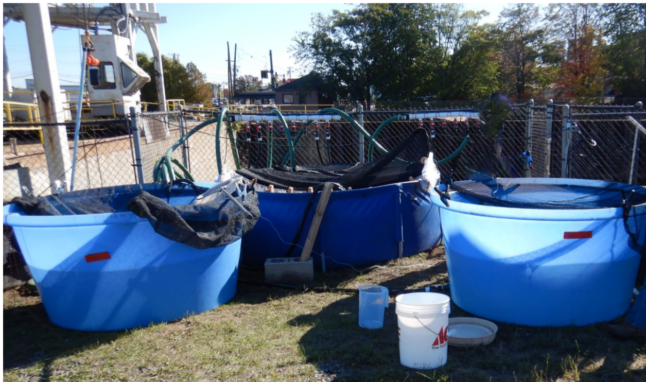
Figure 4-3 Fish pre-test holding facility (center) and post-recapture 48-hour delayed mortality airlift holding tanks.
