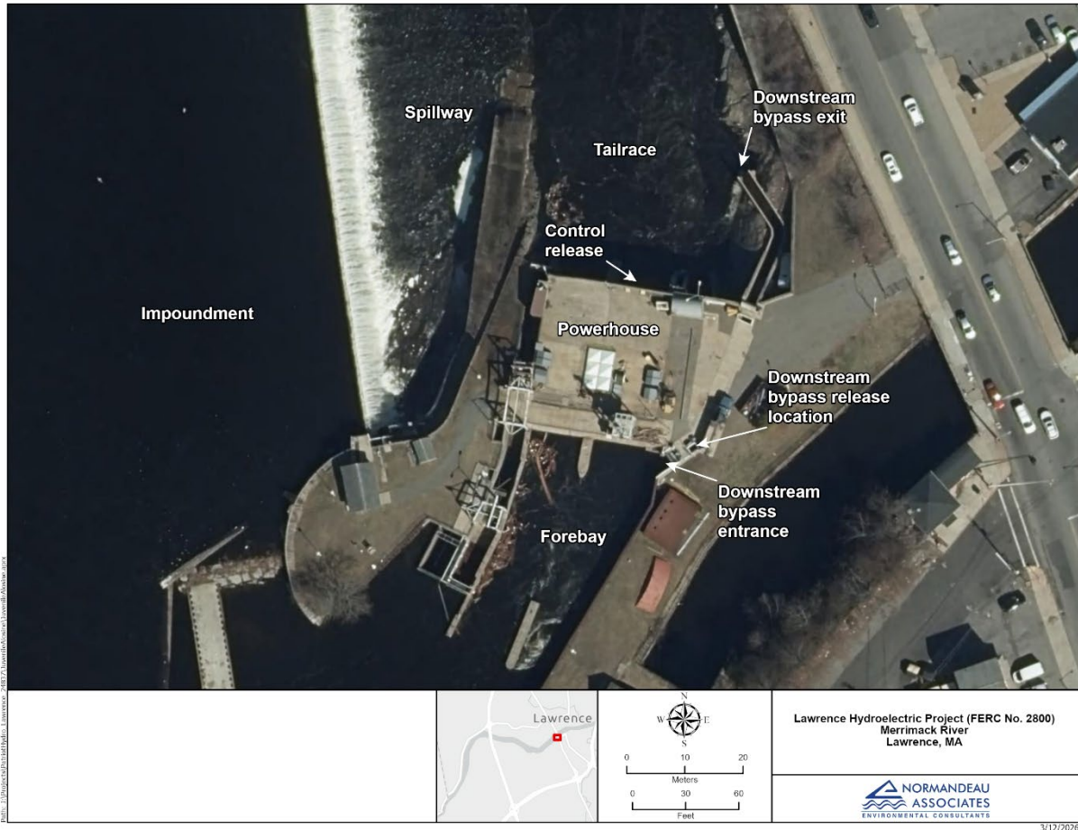
Figure 2-2. Relative location of the downstream bypass entrance, test fish release location, exit, and control fish release location associated with the Downstream Juvenile Alosine Passage Assessment at Lawrence.
