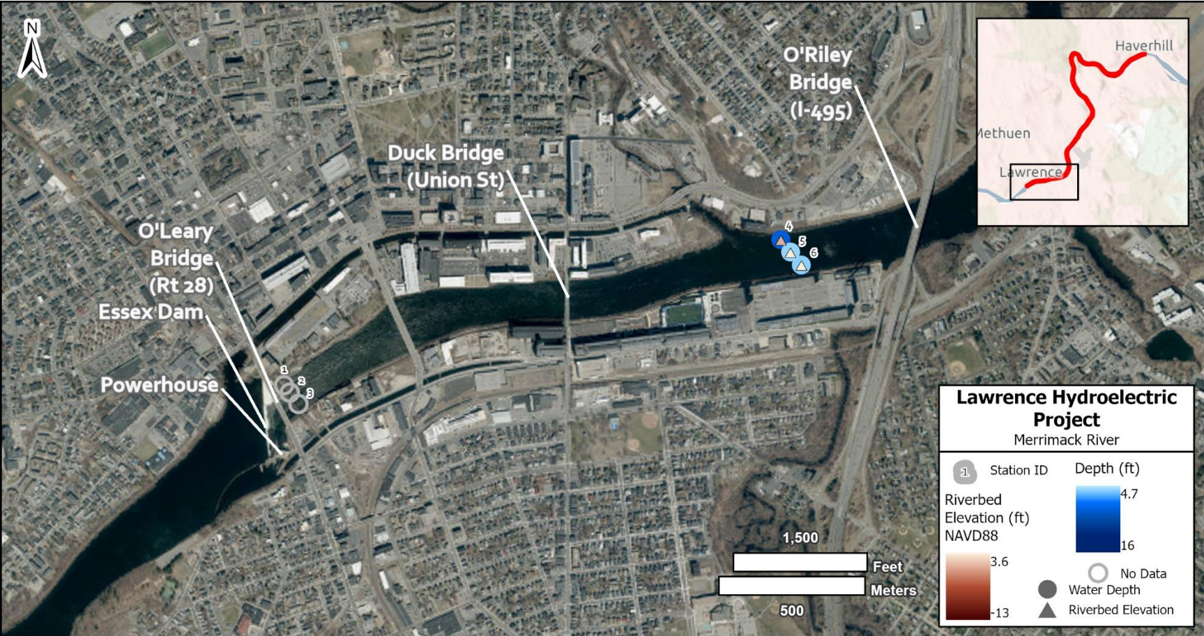
Figure 4-13 Depth and riverbed elevation at Stations 1-6, sampled on July 24, 2025 at the Lawrence Hydroelectric Project on the Merrimack River.
