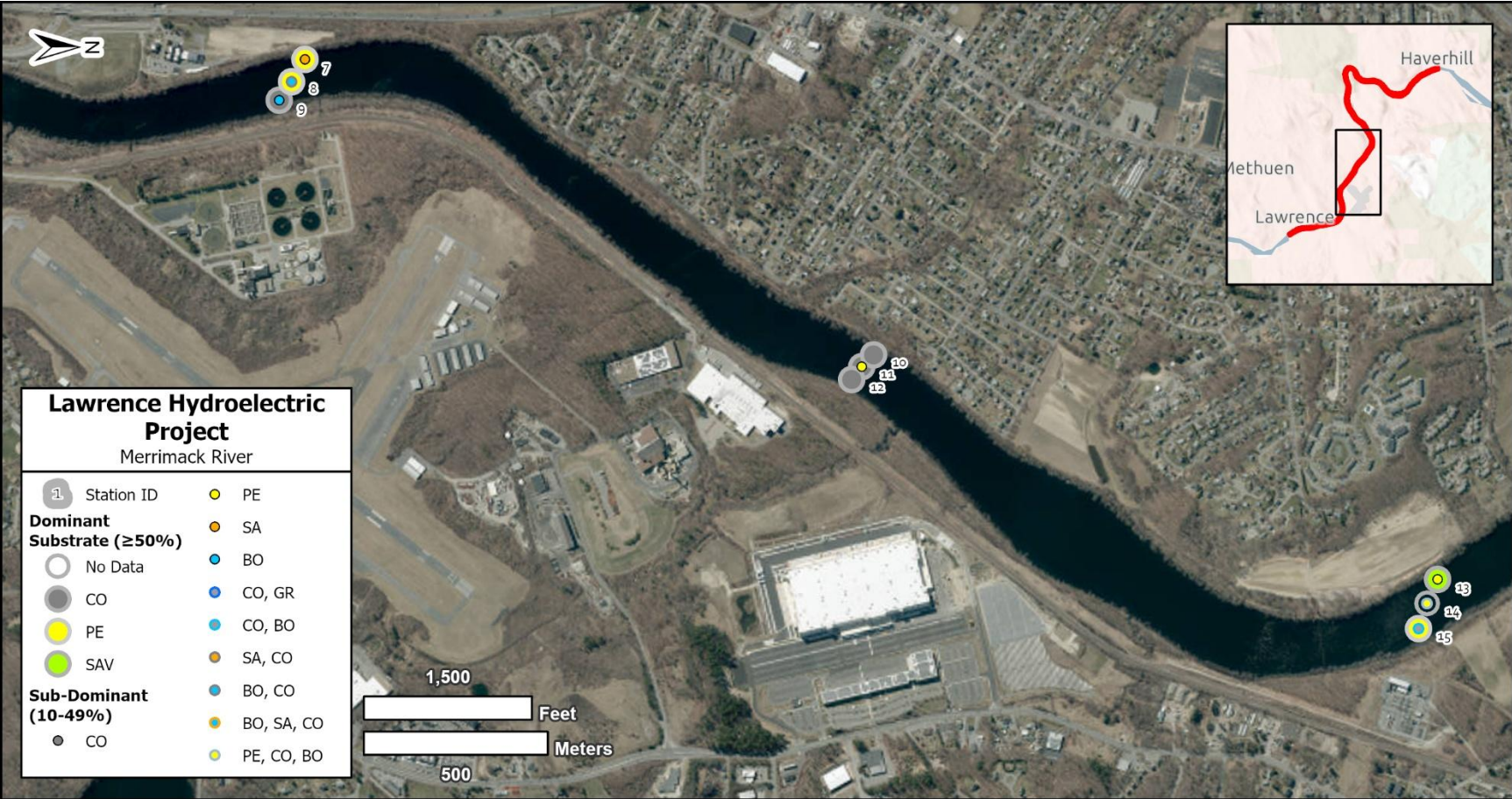
Figure 4-10 Benthic substrates at Stations 7-15, sampled on July 23, 2025 at the Lawrence Hydroelectric Project on the Merrimack River. For substrate classification: BO=boulder; CO=cobble; PE=pebble; GR=gravel; SA=sand; SI=silt; SH=shell; and SAV=submerged aquatic vegetation (primarily eelgrass).
