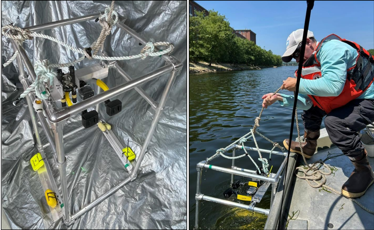
Figure 3-2 Photo of the underwater video frame during mobilization (left) and deployment (right).
