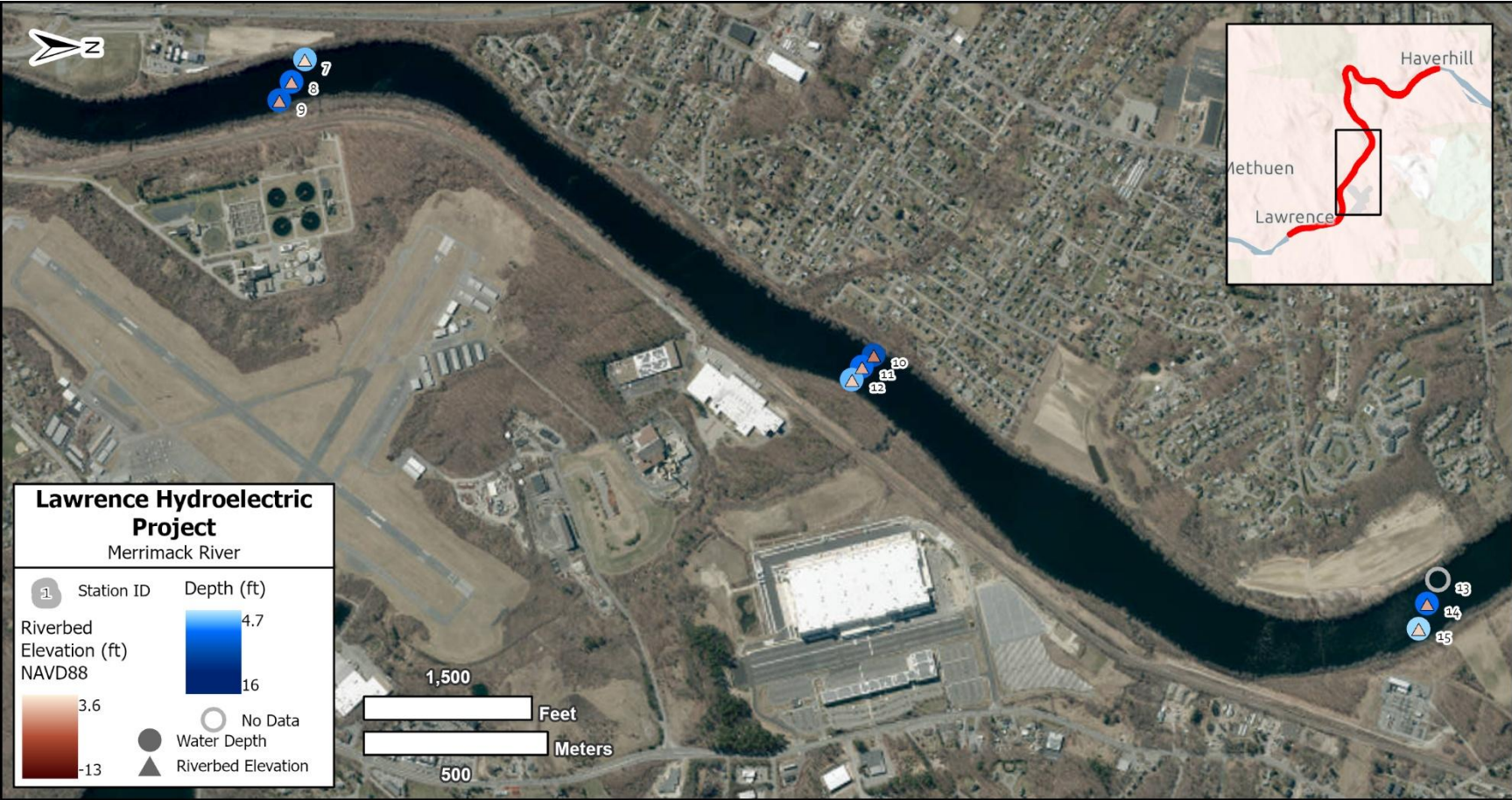
Figure 4-14 Depth and riverbed elevation at Stations 7-15, sampled on July 23, 2025 at the Lawrence Hydroelectric Project on the Merrimack River.
