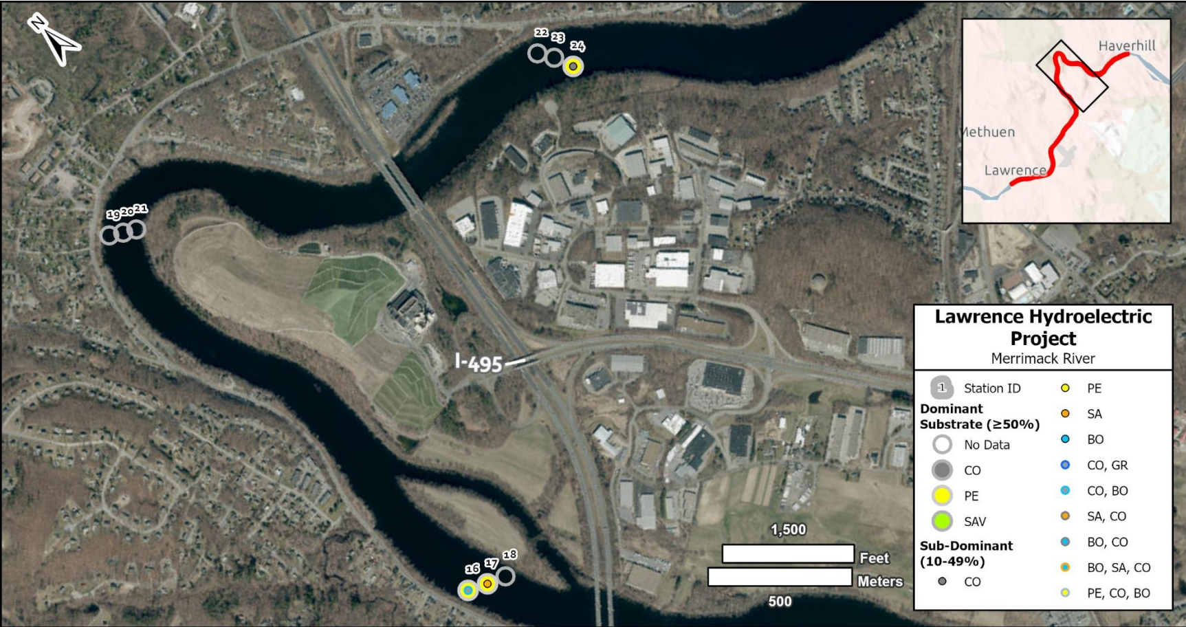
Figure 4-11 Benthic substrates at Stations 16-24, sampled on July 22, 2025 at the Lawrence Hydroelectric Project on the Merrimack River. For substrate classification: BO=boulder; CO=cobble; PE=pebble; GR=gravel; SA=sand; SI=silt; SH=shell; and SAV=submerged aquatic vegetation (primarily eelgrass).
