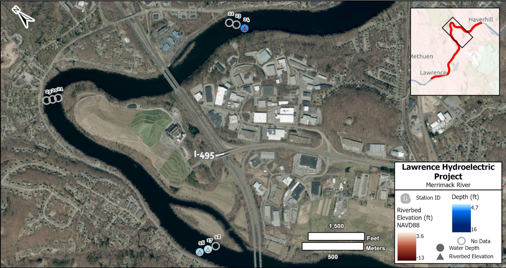
Figure 4-15 Depth and riverbed elevation at Stations 16-24, sampled on July 22, 2025 at the Lawrence Hydroelectric Project on the Merrimack River.
