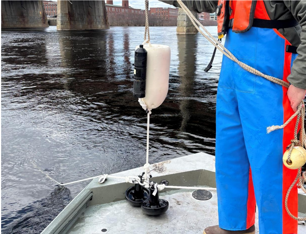
Figure 3-10 InnovaSea VR2Tx submersible autonomous acoustic receiver prior to deployment downstream of Essex Dam.
