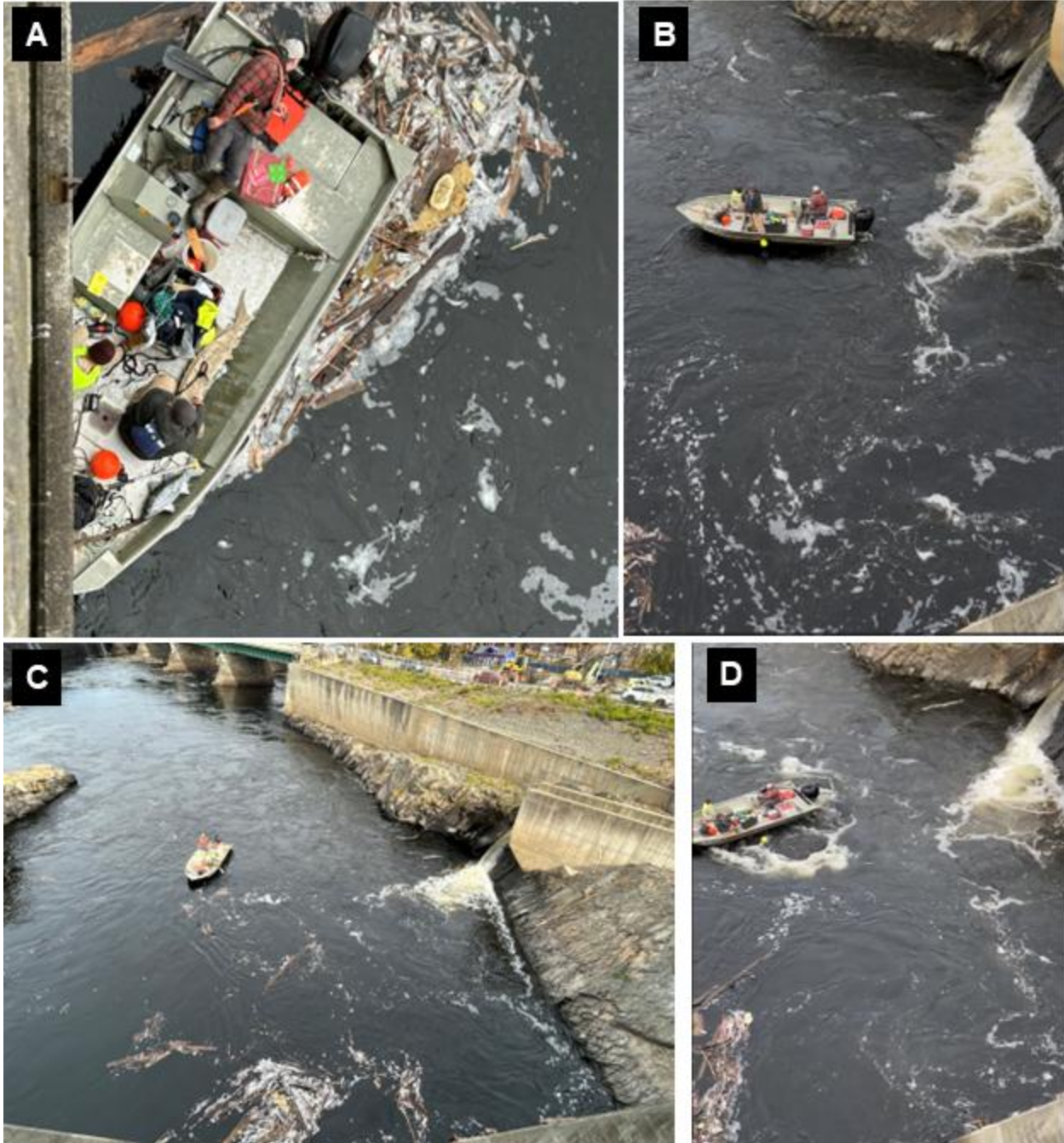
Figure 4-10 Fixed-location monitoring using ARIS and BlueView high-resolution imaging sonars to detect and identify sturgeon within the Project tailrace is not feasible as indicated by the pilot study under controlled conditions due to (A) the high abundance of floating and submerged drift debris; (B-D) entrained bubbles, strong eddies and currents, and upwelling.
