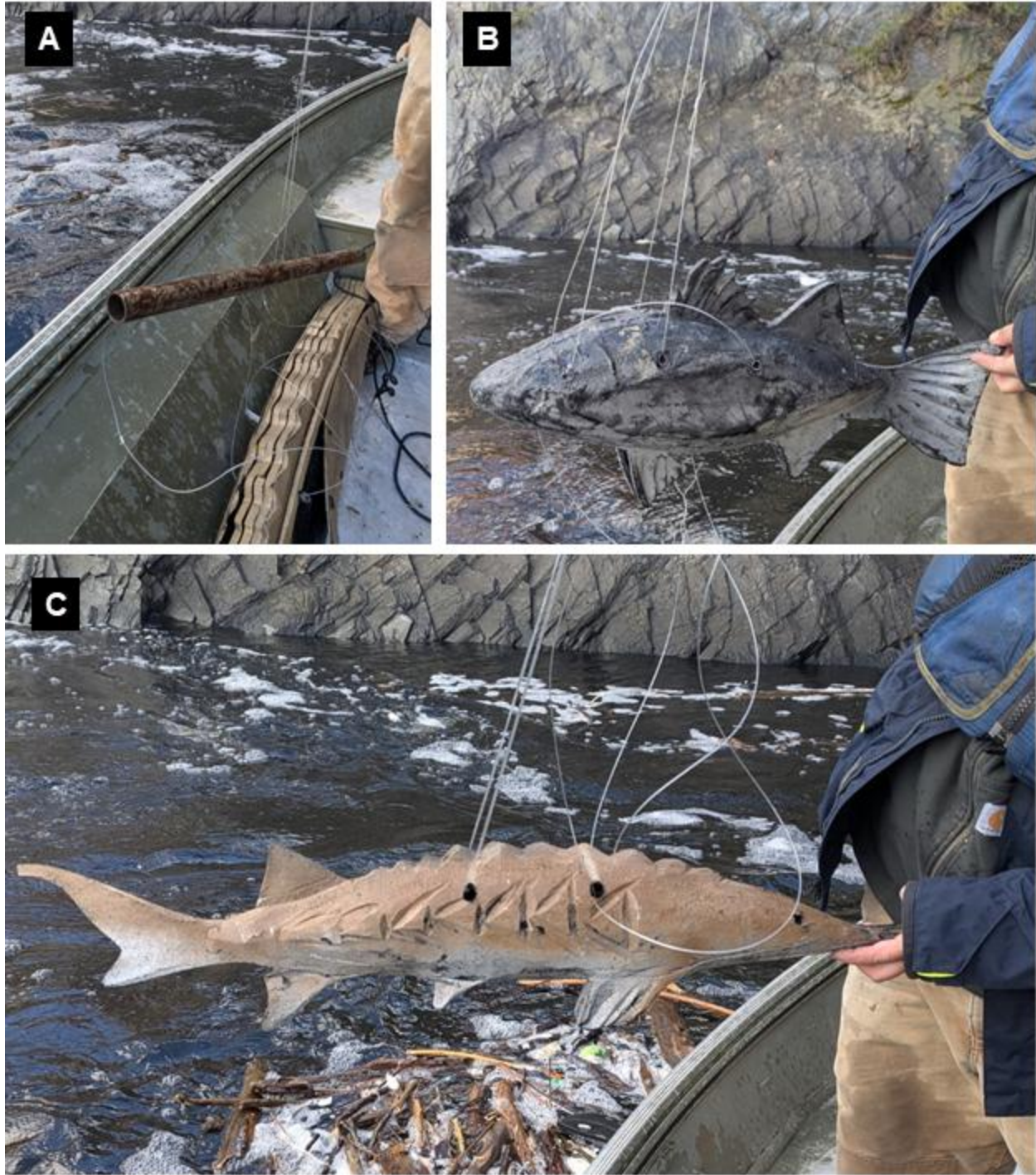
Figure 3-4 Artificial targets for testing detection and identification capabilities of different imaging sonar technologies for fixed-location monitoring of sturgeon in the tailrace at Lawrence Hydroelectric Project: (A) 61-cm long x 3.8-cm diameter steel pipe; (B) 71-cm rubber Striped Bass; and (C) 97-cm rubber sturgeon.
