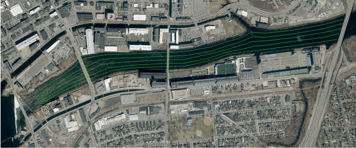
Figure 3-3 The survey area of the Merrimack River for mobile side-scan sonar surveys included nearly bank to bank coverage by five planned lines (green) extending from the I-495 Lawrence Bridge to the boat ramp immediately downriver of the O'Leary Bridge (Route 28) and an old railroad bridge.
