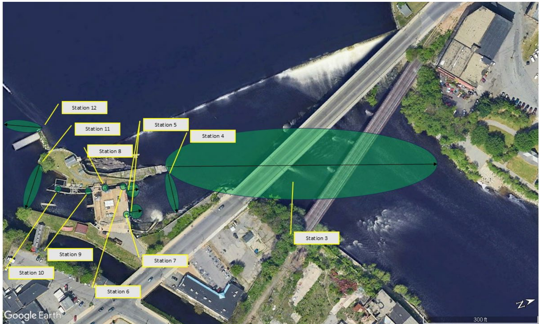
Figure 4-2. Stationary radio telemetry receiver locations associated with the Upstream Anadromous Fish Passage Assessment relative to Essex Dam and the Lawrence powerhouse, spring 2025.
