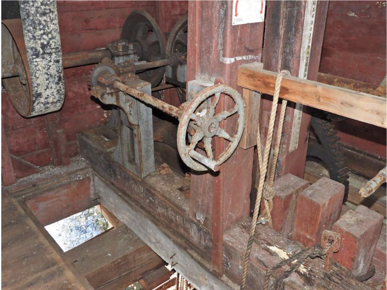
Figure 6-28. Detail of the South Canal Gatehouse manual and electric hoisting systems, and leaf gate stems (lower right); view facing west.
