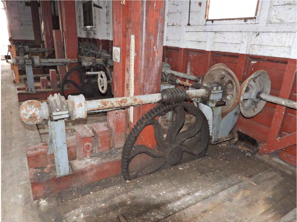
Figure 6-10. Detail of the North Canal Gatehouse gate hoist, view facing south.
