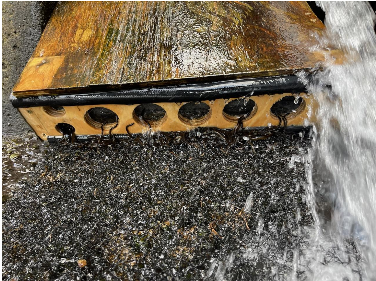
Figure 5-9. Cover used to seal the south side eel ramp during internal efficiency testing.
